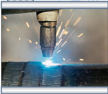
Hardfacing by Rapid Arc.
